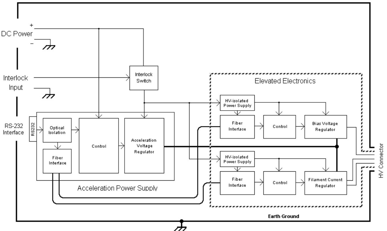
Figure 1. Block Diagram of 3603.
