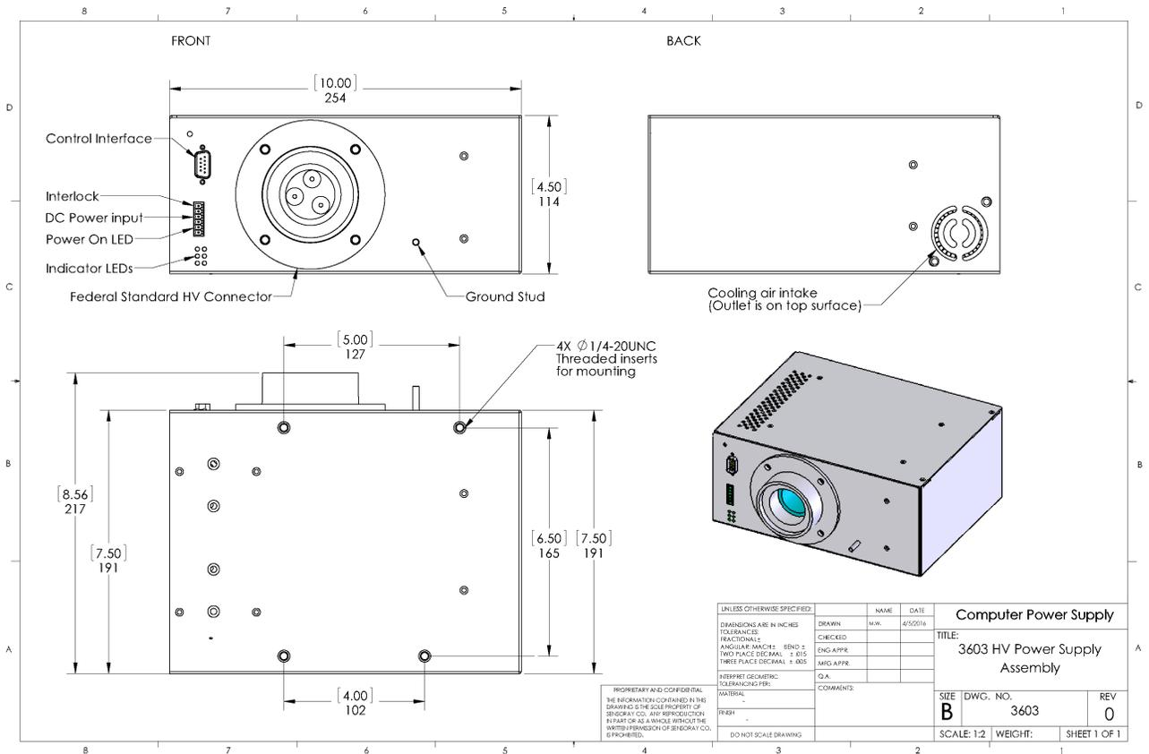
Figure 3. Physical layout and placement of connectors.
