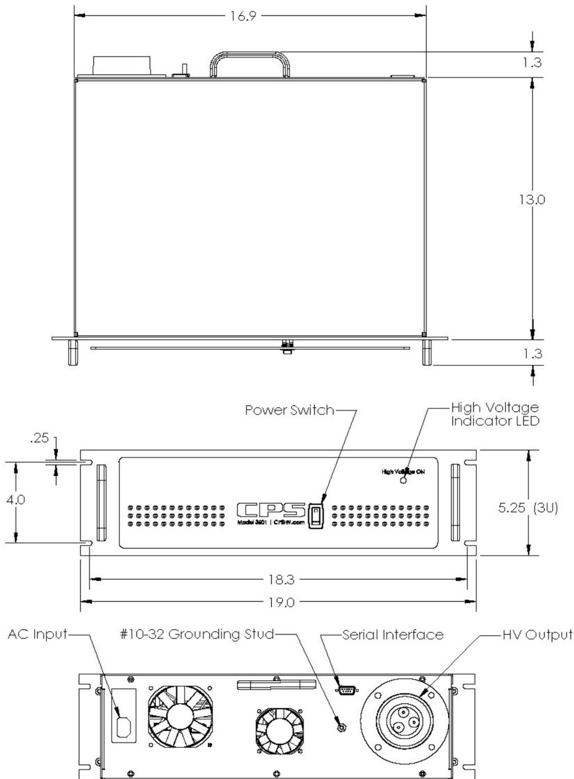
Figure 3. Physical layout and placement of connectors.
